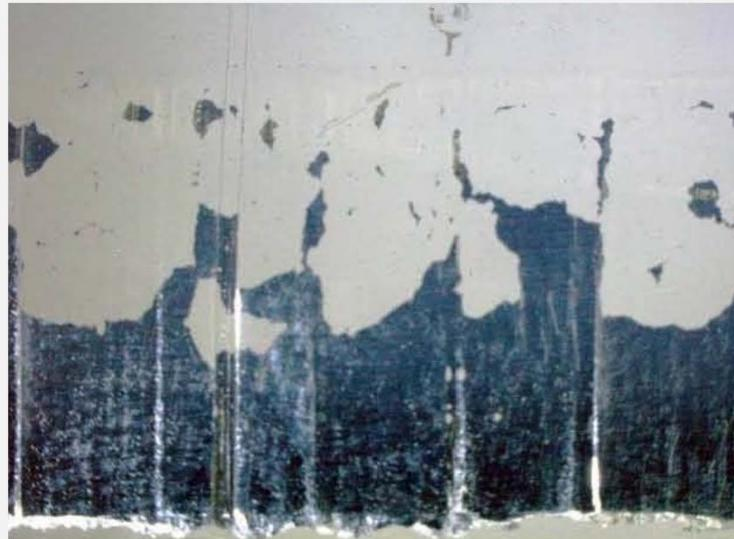
Film metallization displaying significant corrosion
